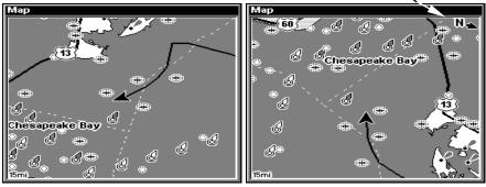
Map orientation is shown in north up (left) and track up (right).
